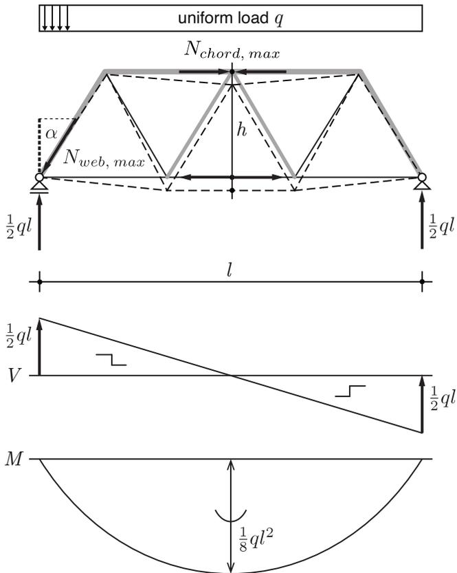
Figure 14.6: Load distribution in a truss
