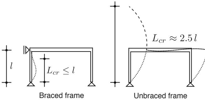
Figure 15.7: Buckling length
