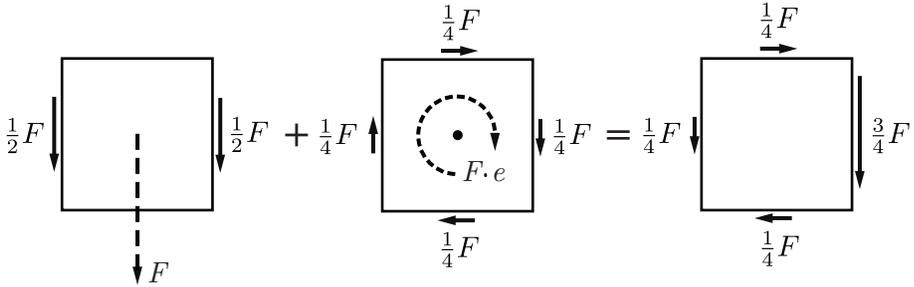
Figure 19.10: Centric force and torsion couple
