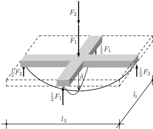
Figure 14.4: Load distribution in a two-way spanning floor slab
