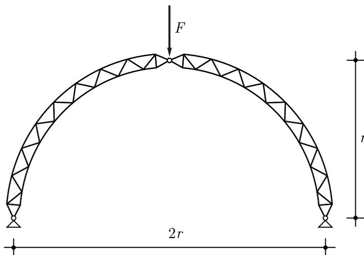
Figure 20.5: Three-hinged truss arch
