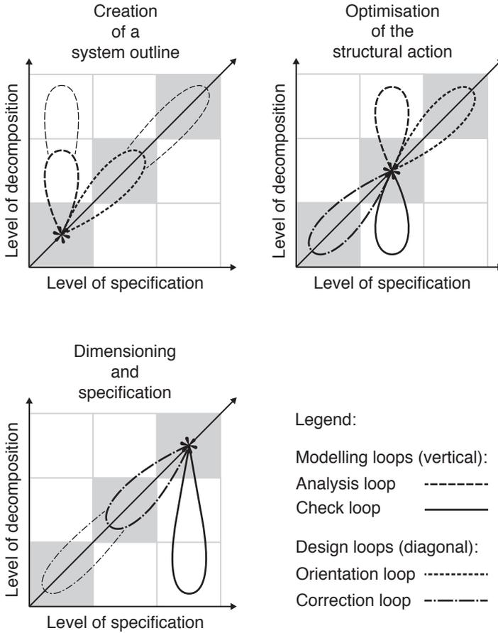
Figure 10.7: Structural design loops
