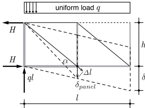
Figure 15.4: Shear deformation in a cantilevered truss
