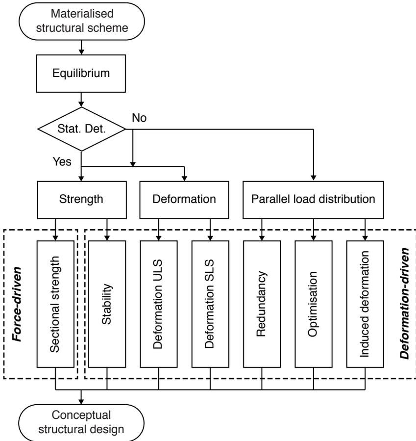
Figure 12.2: Force and deformation-driven parameters
