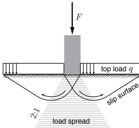
Figure 15.11: Failure mechanism of a spread foundation
