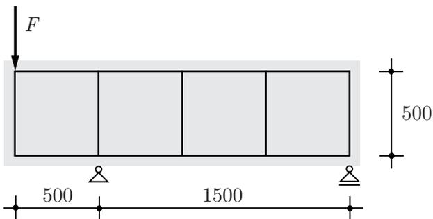
Figure 21.1: Cantilevered reinforced concrete beam
