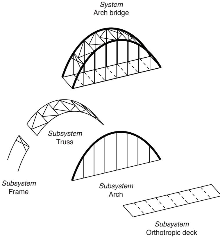
Figure 9.1: Assembly of an arch bridge
