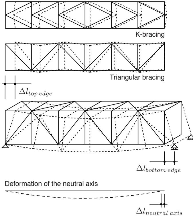
Figure 14.14: Induced deformation in a truss bridge
