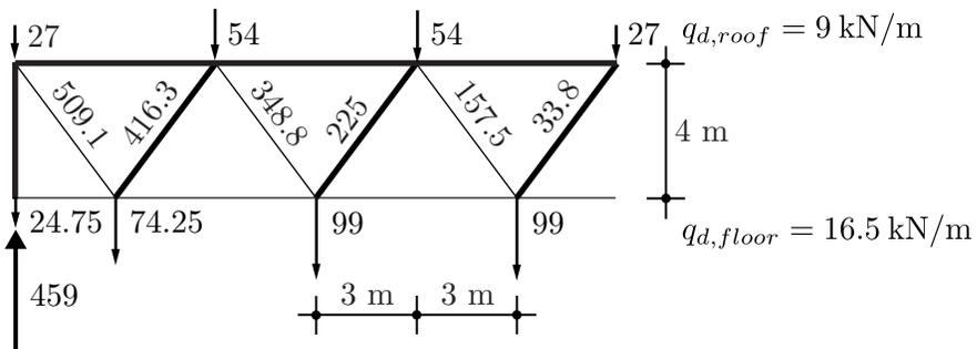
Figure 20.3: Truss load distribution web members
