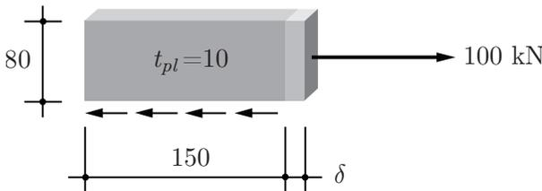
Figure 14.11: Axial deformation of the stiffener
