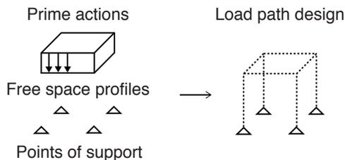
Figure 13.1: Load path design
