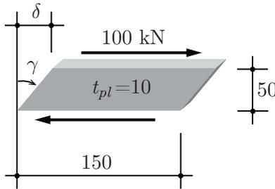
Figure 14.12: Shear deformation of the stiffener
