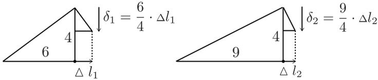
Figure 18.3: Deformation of the ties
