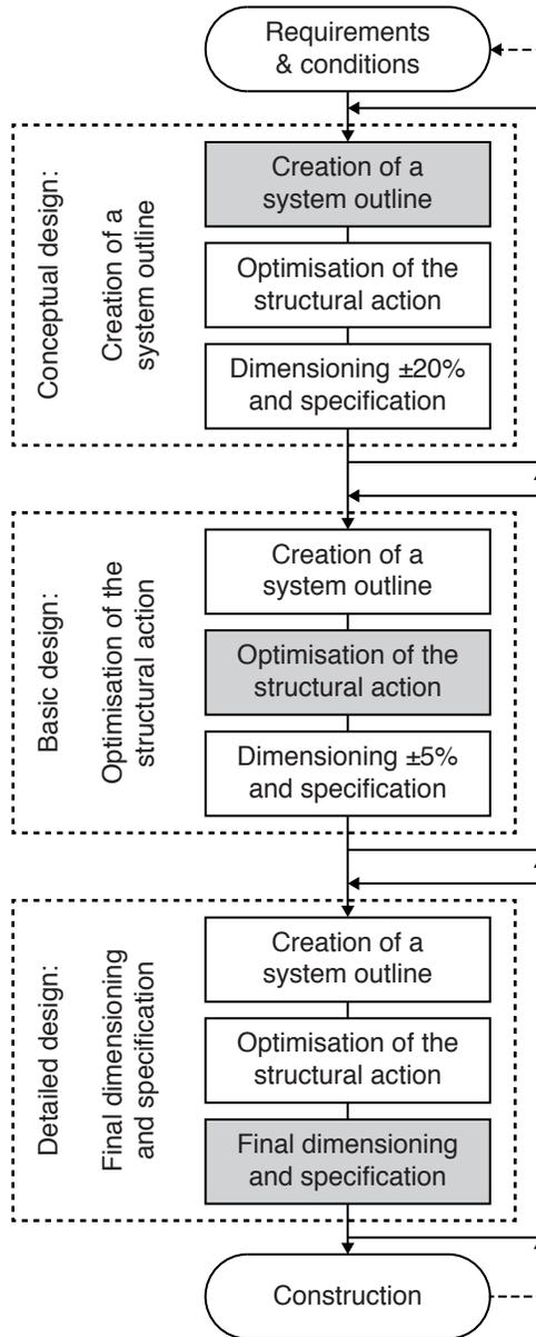
Figure 8.4: Fundamental structural design process
