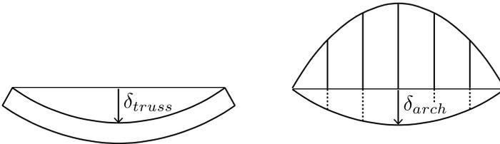
Figure 20.2: Displacement combined truss girder and tied arch
