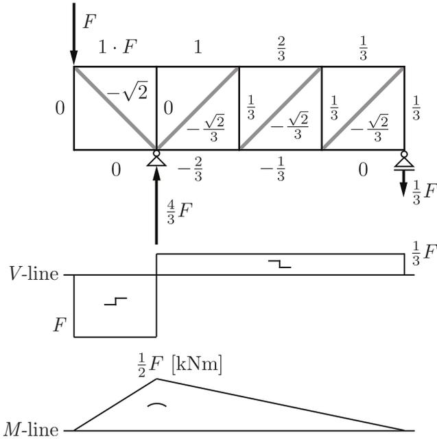
Figure 21.2: Load distribution concrete beam
