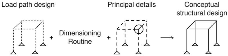
Figure 13.5: Conceptual structural design
