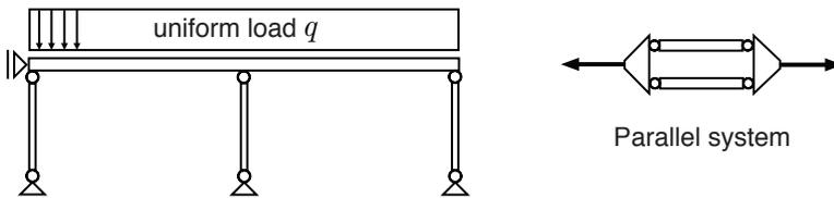
Figure 14.2: Statically indeterminate structure
