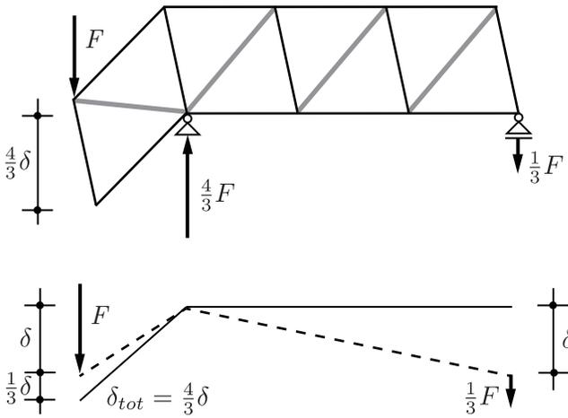
Figure 21.5: Displacement of the cantilever
