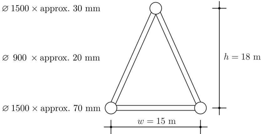
Figure 17.9: Truss dimensions
