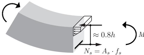
Figure 15.9: Bending strength of a concrete member
