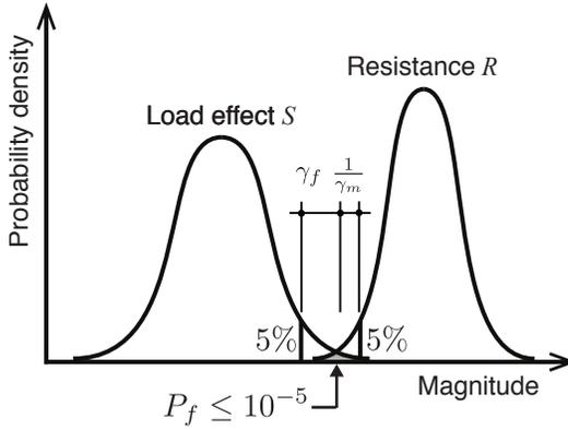
Figure 3.1: Structural safety Eurocode
