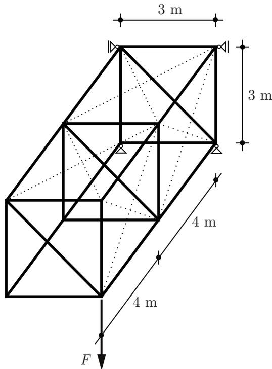
Figure 19.7: 3-D square box truss with eccentric loading
