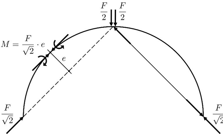
Figure 20.6: Load distribution three-hinged arch
