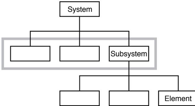
Figure 9.2: Subsystem level
