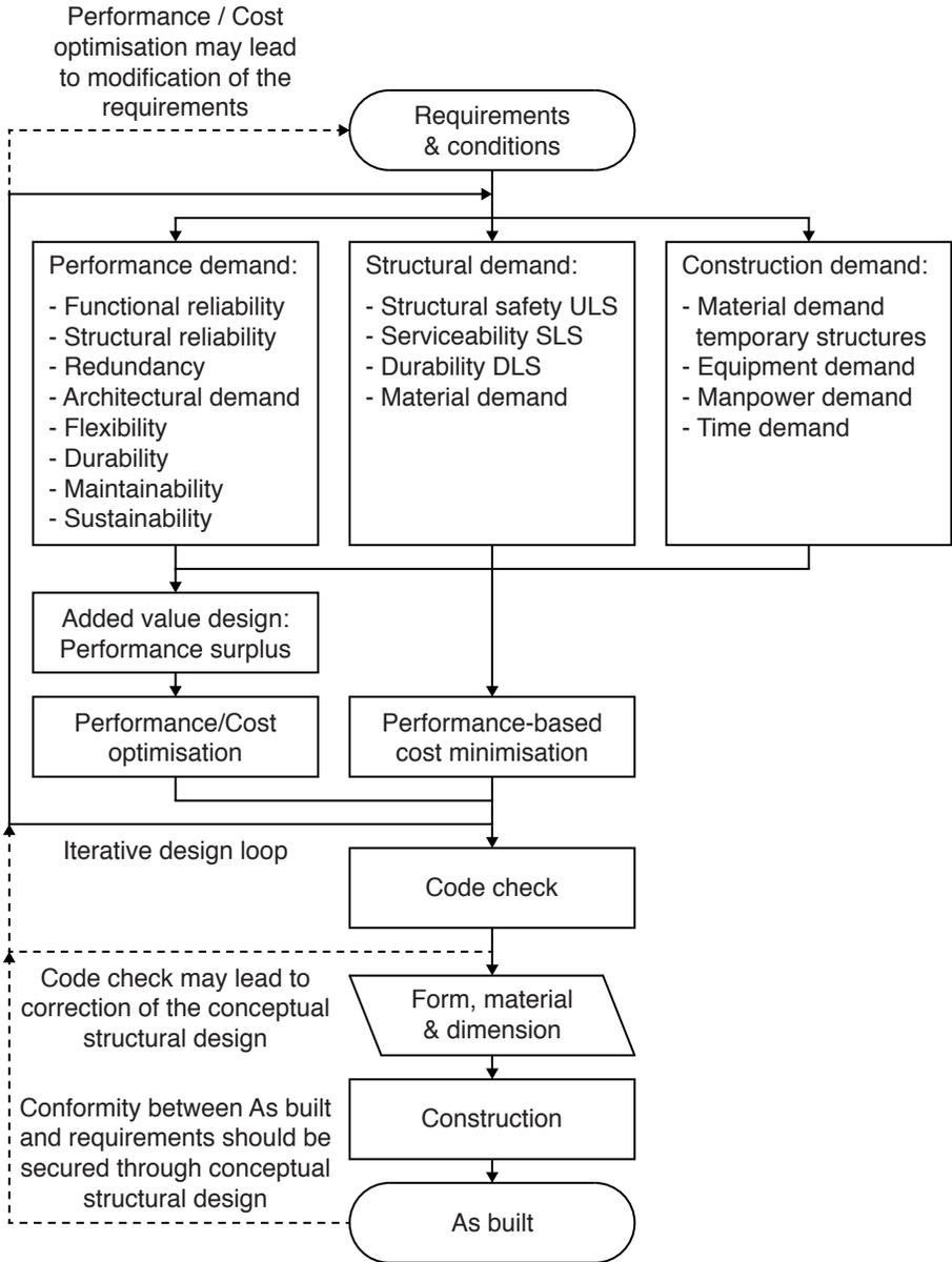
Figure 7.1: Conceptual structural design process
