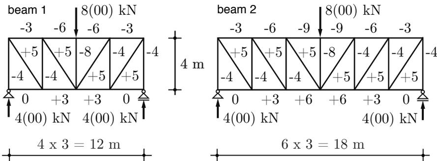
Figure 19.3: Load distribution 2-D trusses
