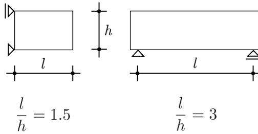
Figure 15.3: Transition slenderness for stocky to slender beams
