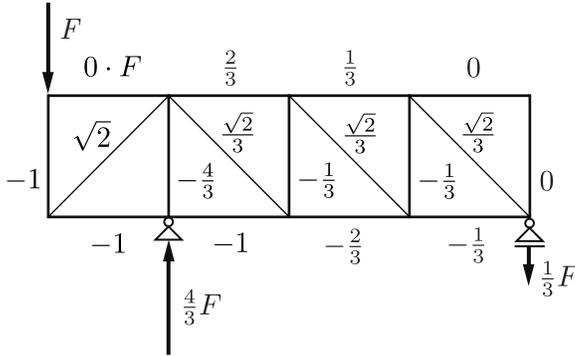
Figure 21.10: Load distribution truss analogy
