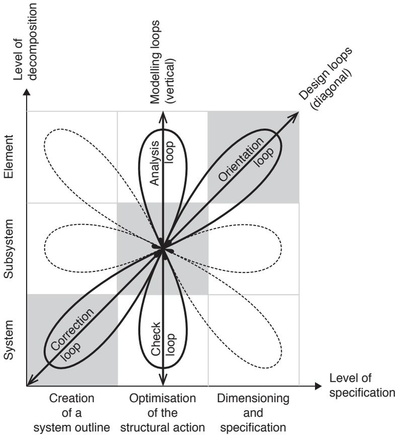
Figure 10.6: Fundamental structural design loops
