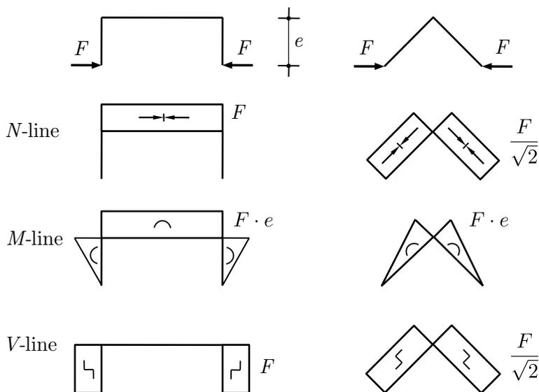
Figure 20.7: N-, M-, and V-lines of enclosing simplified structures
