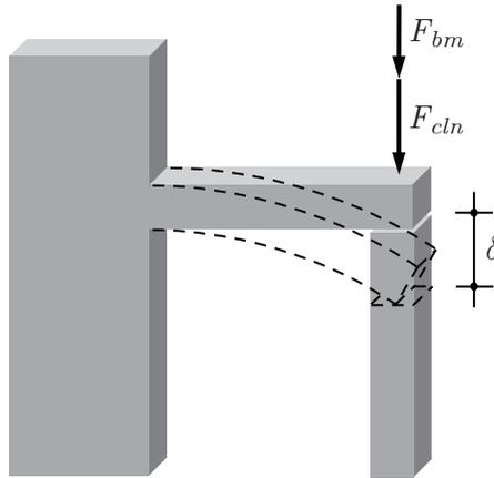
Figure 14.3: Parallel bending and axial force
