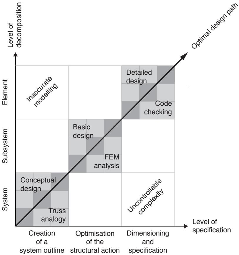
Figure 10.4: Structural design path
