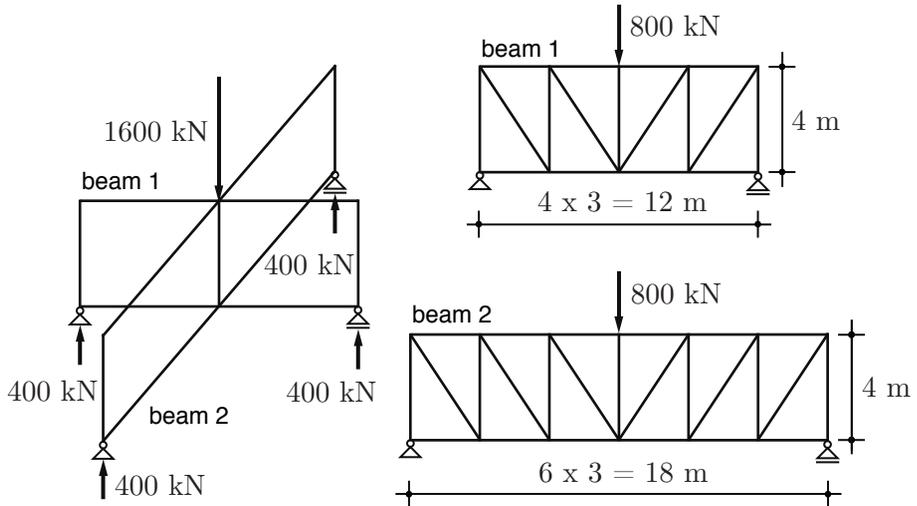
Figure 19.1: Bracing system with trusses
