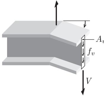
Figure 15.1: Shear strength
