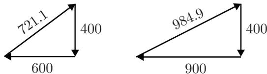
Figure 18.2: Load distribution 2-D struts and ties
