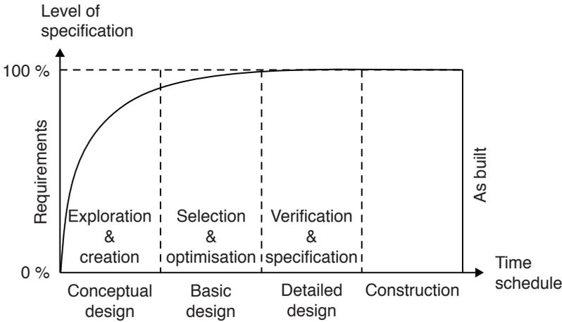
Figure 8.3: Level of specification
