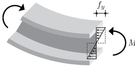
Figure 15.10: Bending strength of a steel member
