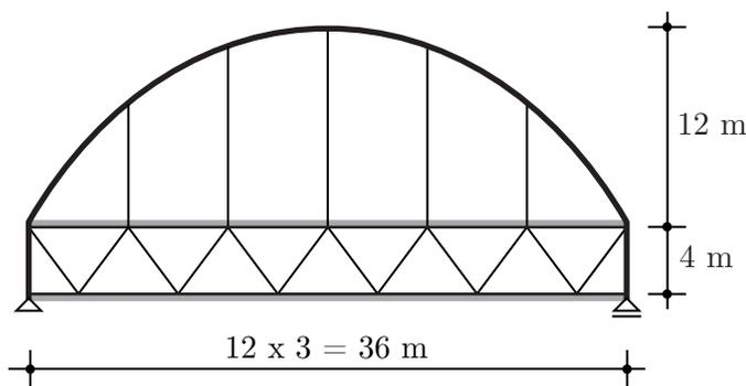
Figure 20.1: Truss girder bridge building combined with tied arch
