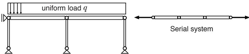
Figure 14.1: Statically determinate structure
