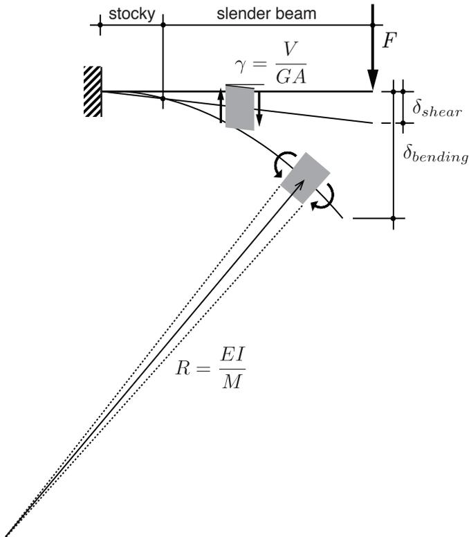
Figure 15.2: Bending and shear deformation
