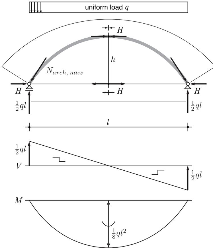
Figure 14.7: Load distribution in an arch
