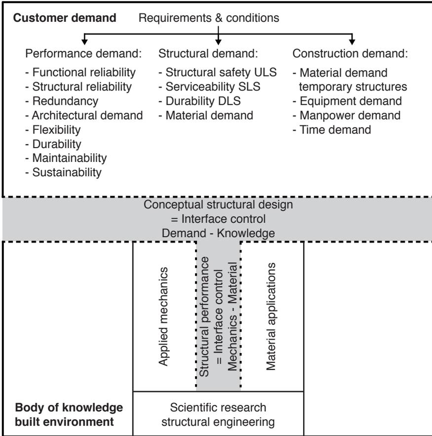
Figure 4.1: Structural design as an interface control approach
