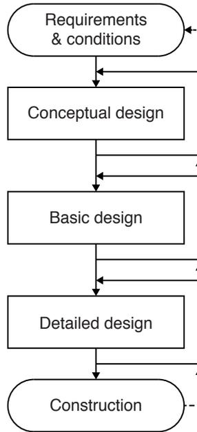
Figure 8.1: Structural design process
