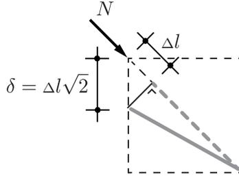
Figure 21.3: Shear deformation of the cantilever
