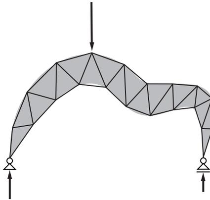
Figure 13.2: Truss-analogy in load path design
