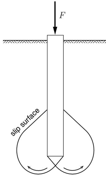
Figure 15.12: Failure mechanism of a pile foundation
