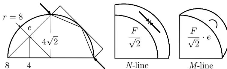
Figure 20.8: N- and M-lines of a semi-circular arch
