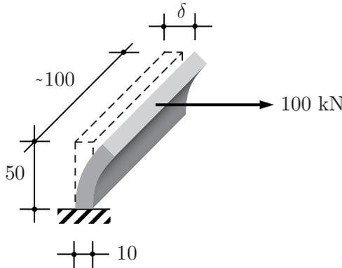
Figure 14.10: Bending deformation of the flange
