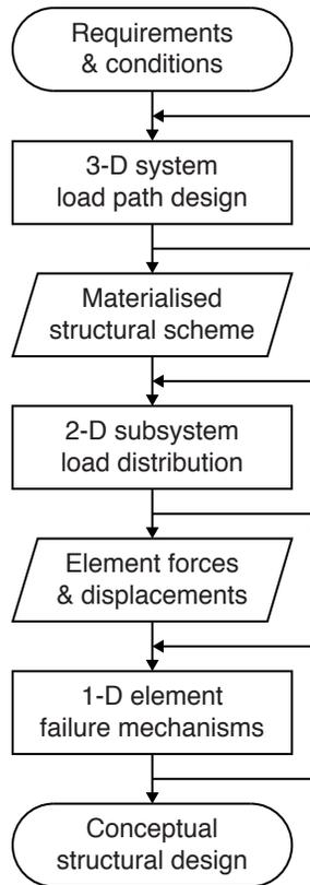
Figure 12.3: Dimensioning routine of the conceptual structural design
