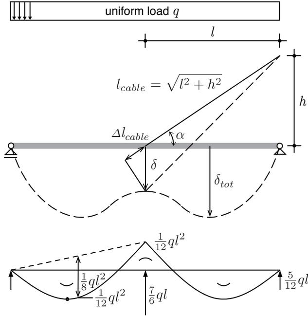
Figure 14.5: Redistribution in a cable-stayed beam
