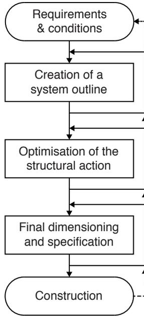
Figure 8.2: Fundamental structural design cycle
