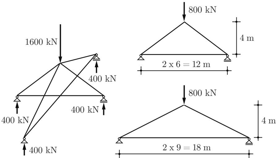
Figure 18.1: Bracing system with struts and ties
