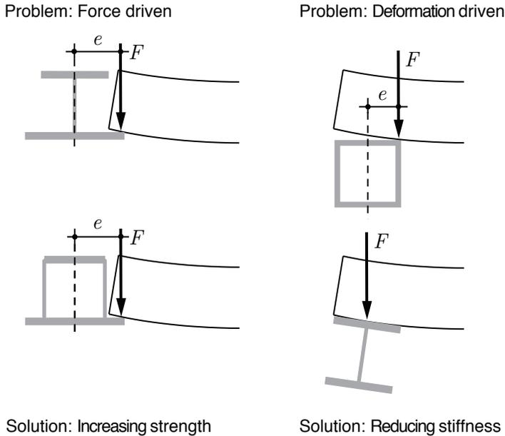
Figure 14.13: Induced deformation torsional clamped beam
