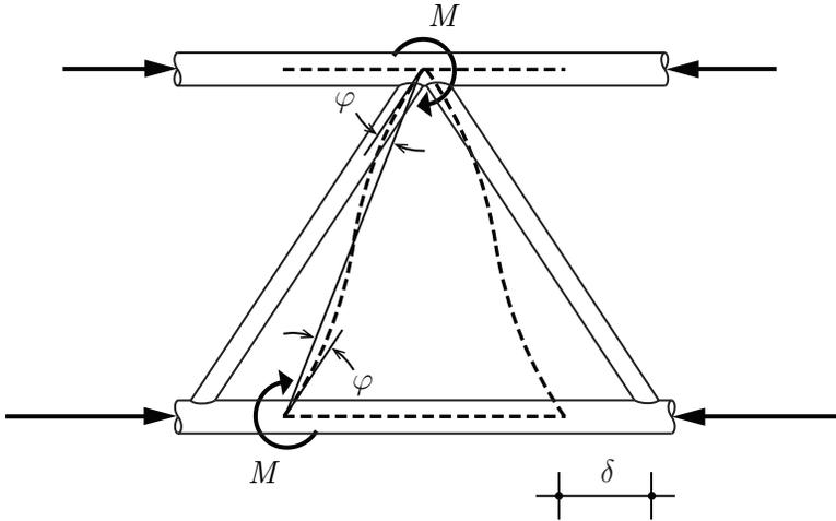
Figure 17.8: Induced deformation of the Maeslant storm surge barrier
