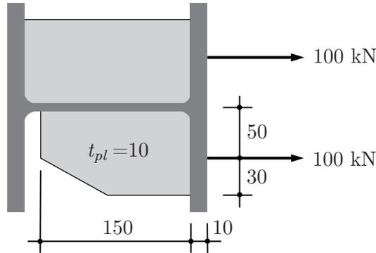
Figure 14.9: Stiffener plate in a beam-to-column joint
