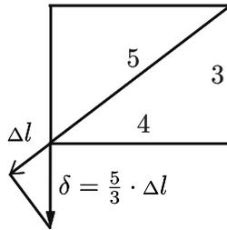
Figure 19.9: Displacement due to the elongation of a bar
