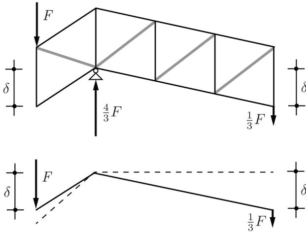
Figure 21.4: Contribution shear deformation right span
