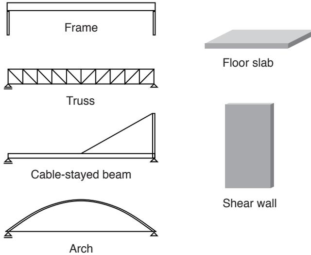
Figure 9.3: Basic structural forms
