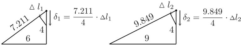
Figure 18.4: Deformation of the struts
